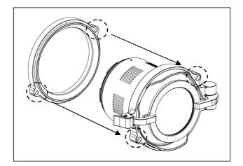
2. Insert holder B from the rear side of the port, align the openings on A and B.
