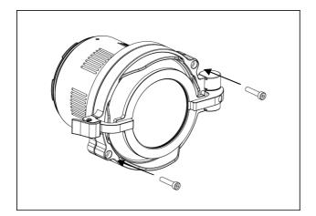
3. Fasten the flip diopter holder onto the port by the screws provided.
