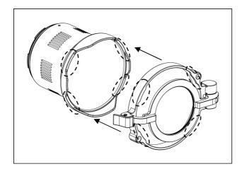
Align the four bayonets of holder A with the recessed parts of the port shade as indicated on the diagram. Gently place holder A on the front of the lens port.
