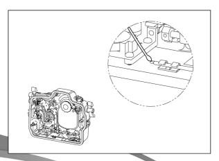
2. Test the moisture alarm by contacting the two wires near the bottom of the housing with a damped cotton bud; the alarm should start giving out a repeating "beep" sound along with a flashing red light. The "beep" sound and the light should keep on going for 5 seconds after the removal of the damped cotton bud.
