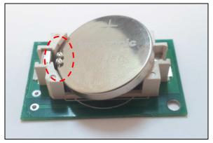
1. Install the CR2450 battery provided into the battery compartment inside the rear housing. Then switch on the alarm.
