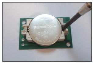
To remove the battery, use a small flat-head screwdriver to lift up the battery as shown.
