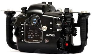
The 5D Mark III Live View/Movie Switch is placed at the right thumb, allowing quick changes between shooting modes. A lever accessing ISO is also located for fingertip control at the right thumb. ISO is exceptionally important when shooting movie clips with a digital SLR as the primary exposure control, and easy access allows quick exposure changes.
