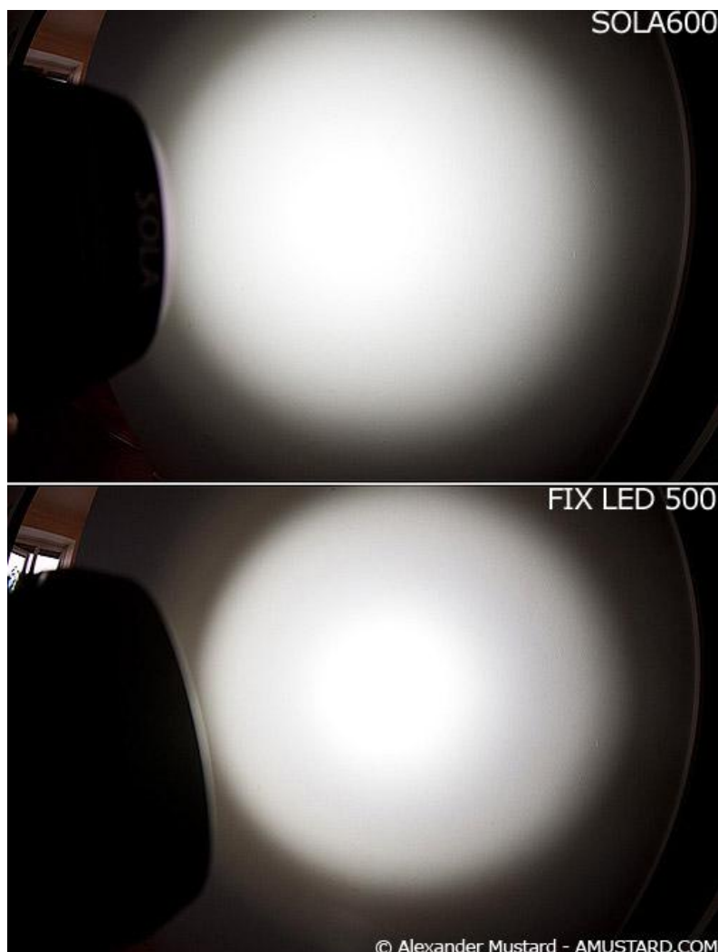
Comparison of light output of SOLA600 (top) and my FIX LED 500 (bottom). Light spots on wall, photographed with fisheye lens. SOLA600 produces a wider and softer pool of light, but both are impressive performers.
